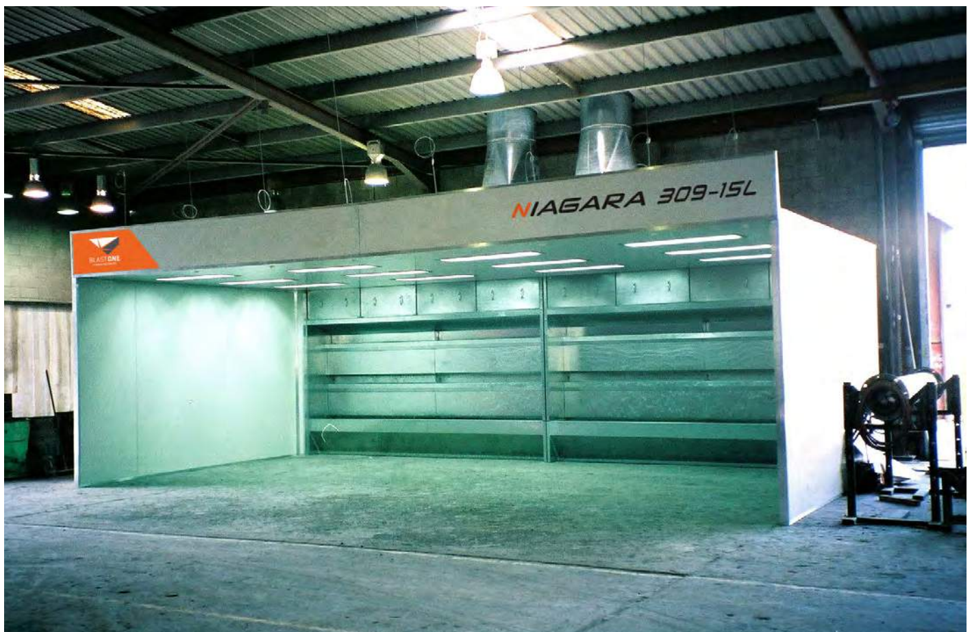
OPEN FACED WATER WASH BOOTH USED FOR GRINDING APPLICATIONS
