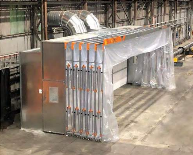
OPEN FACED MASTRE-FLEX BOOTH RETRACTED
