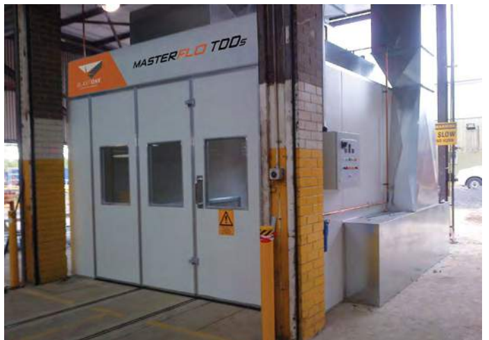
SIDE DOWN-DRAFT SPRAY BOOTH/CURING OVEN
