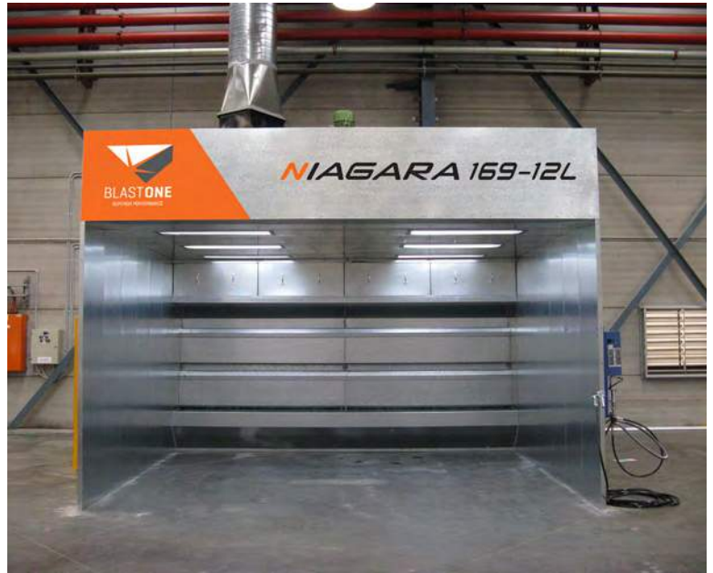
OPEN FACED WATER WASH BOOTH USED FOR HIGH VOLUME FURNITURE PAINTING
