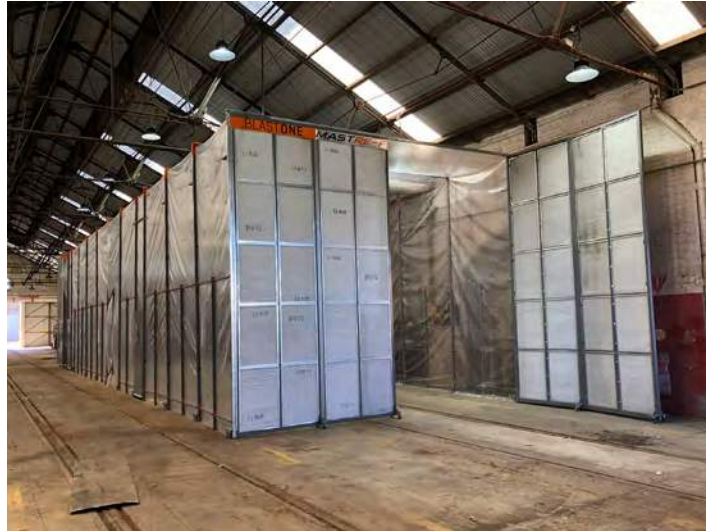
ENCLOSED MASTRE-FLEX BOOTH EXTENDED - WITH DOOR OPEN
