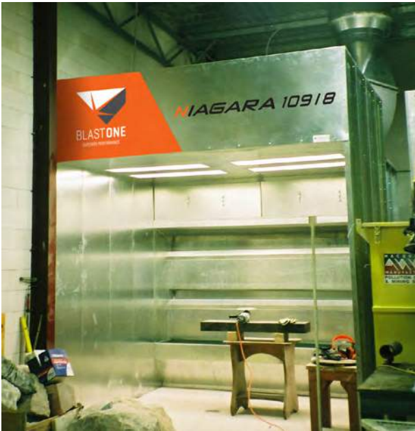
OPEN FACED WATER WASH BOOTH USED FOR STONE MASONRY WORK
